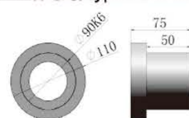
2型丝杆螺母/Type 2 screw nut
